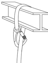
The Tracpac high-abrasion shock-absorbing lanyard with 5,000-lbs. (22.2 kN) gate load carabiner is composed of a shock absorber to which a 1 $\frac{1}{16}$ -in. (30 mm) high-abrasion web lanyard is attached. With a triple action gate loading mechanism, the 5,000-lbs. (22.2 kN) all direction carabiner allows the user the ability to tie back directly to the lanyard arm itself creating a 5,000-lbs. (22.2 kN) structural anchorage connection.
