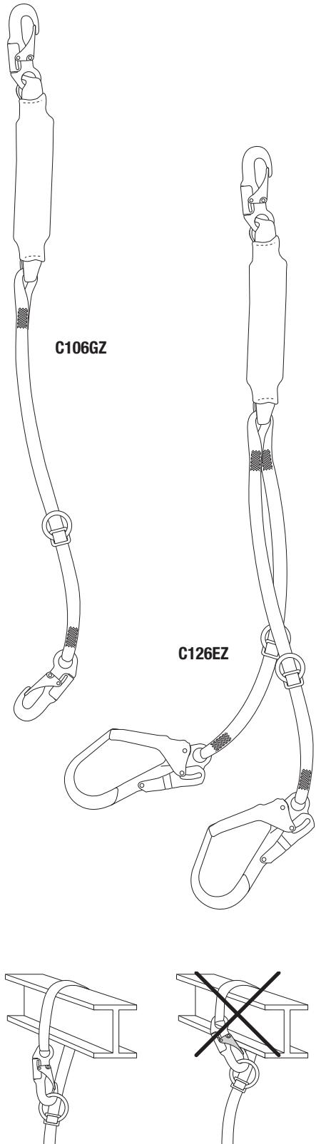
The Tracpac tie-back high-abrasion shock-absorbing lanyard is composed of a shock absorber to which a 1½-in. (30 mm) high-abrasion web lanyard with sliding O-ring is attached. The sliding O-ring allows the user to safely connect the lanyard back on itself (tie-back) for choking on poles, beams, etc.
